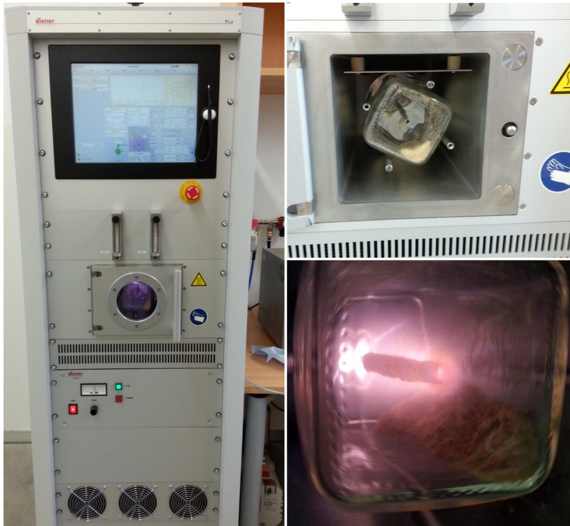
Figure 3.5 Low pressure plasma system PICO from DIENER ELECTRONIC GmbH and details of the plasma chamber with the squared section glass bottle (sample holder).
