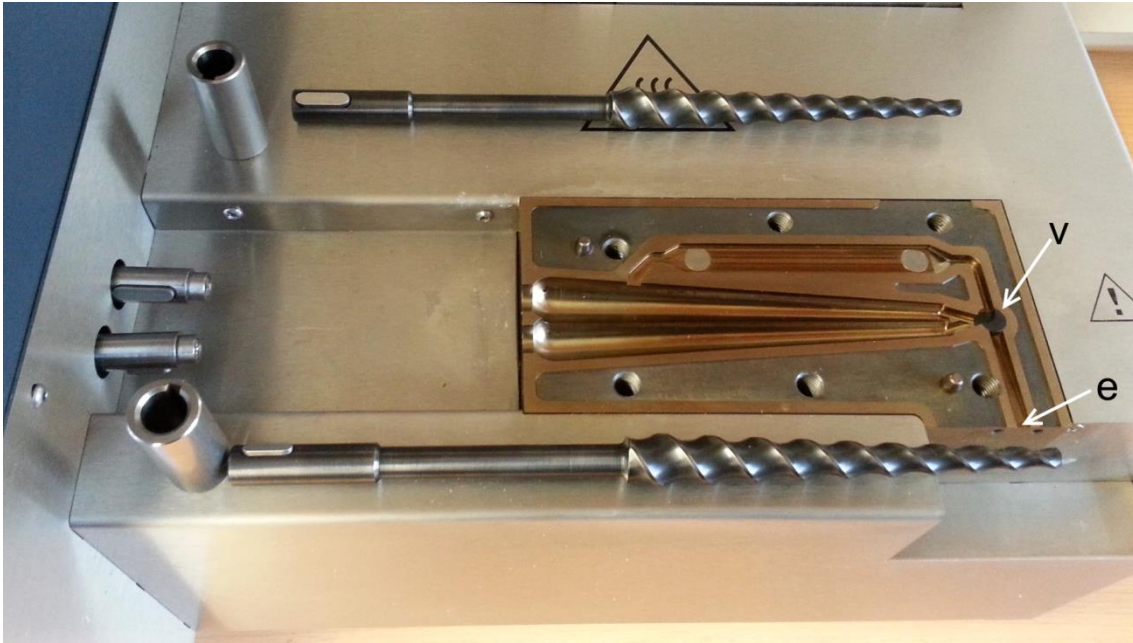
Figure 3.7 – Mixing chamber with capillary channel and screws of the HAAKE MINI-LAB micro-extruder. “v” indicates the valve that controls the melted material flux and “e” indicates the exit opening.
