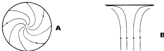
Figure 2.4: Cross section view (A) and side view (B) of the streamlines for the RDE system. Adapted from [2].
