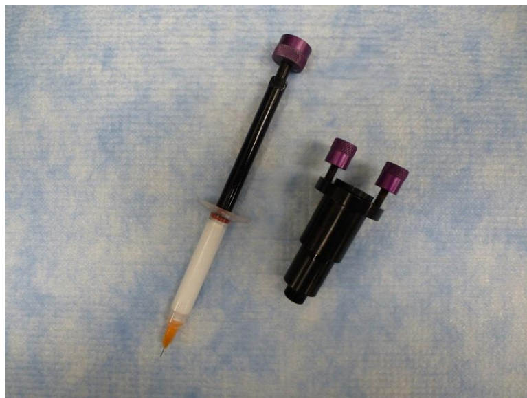
Figure 4.5: Ink placed into the robocasting system syringe. The ink placed in the syringe is the BCMP one.
