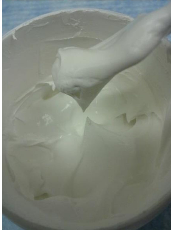
Figure 4.2: \beta -TCMP ink consistence. Notice the stiff peak formed once a spatula is pulled straight up out of the ink.
