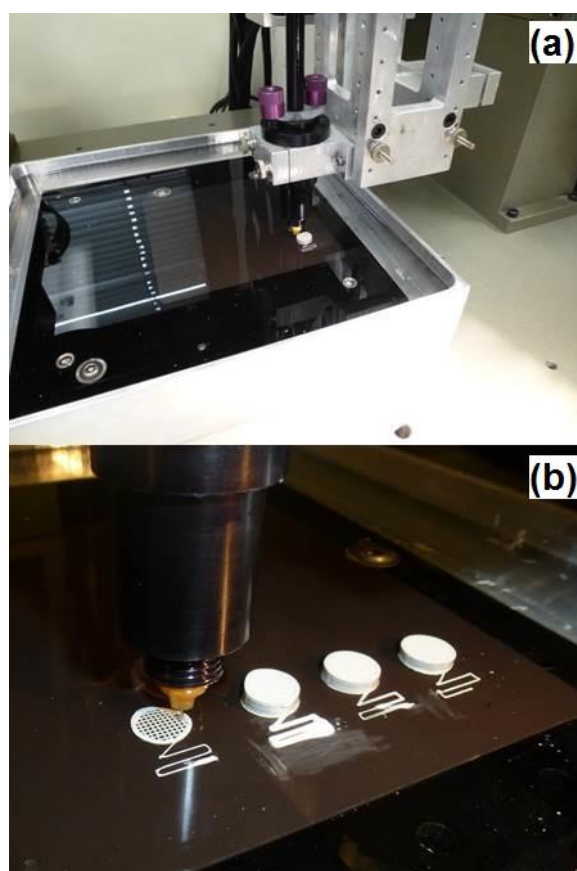
Figure 4.6: (a) direct-write assembly of a BCMP scaffold performed in a non-wetting oil bath; (b) close-up image of the ink deposition.
