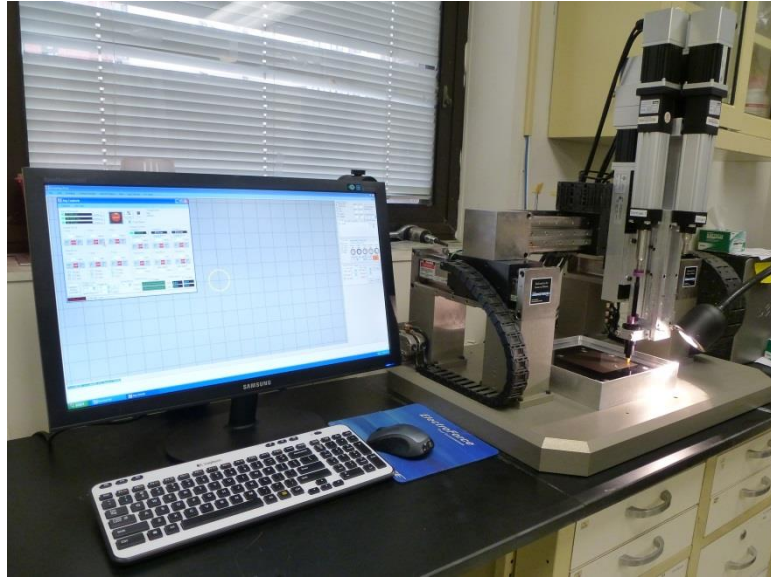
Figure 4.3: Robotic deposition device Aerotech 3200.
