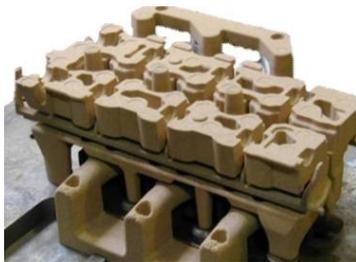
*Figure 2 – Complete set of cores (organic binder)<sup>2</sup>*
