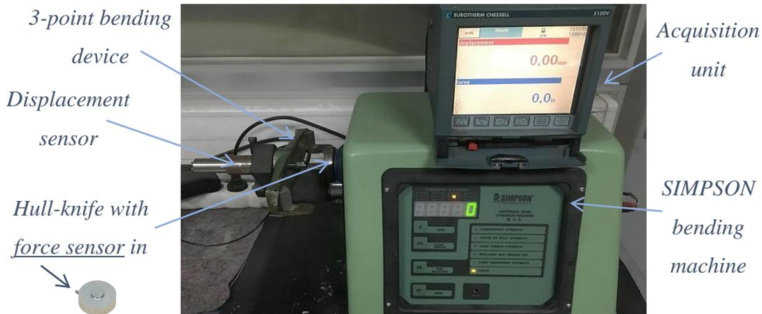
Figure 17 – Assembly of force and displacement sensors on the bending machine
