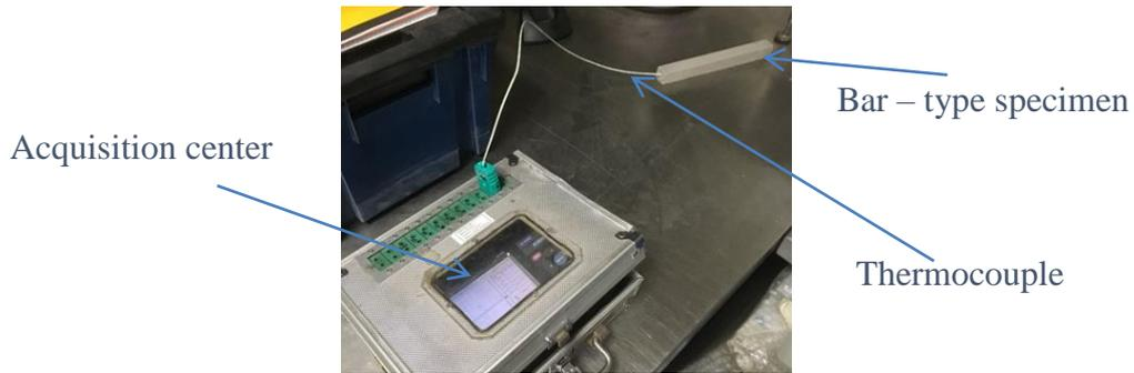
Figure 13 - Instrumentation of a bar-type specimen used in the bending tests
