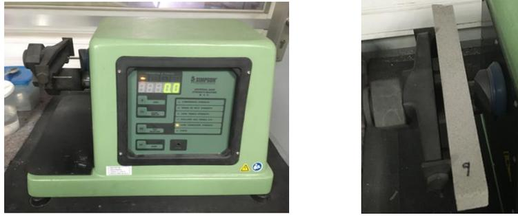
*Figure 15 – SIMPSON 3-point bending machine*
