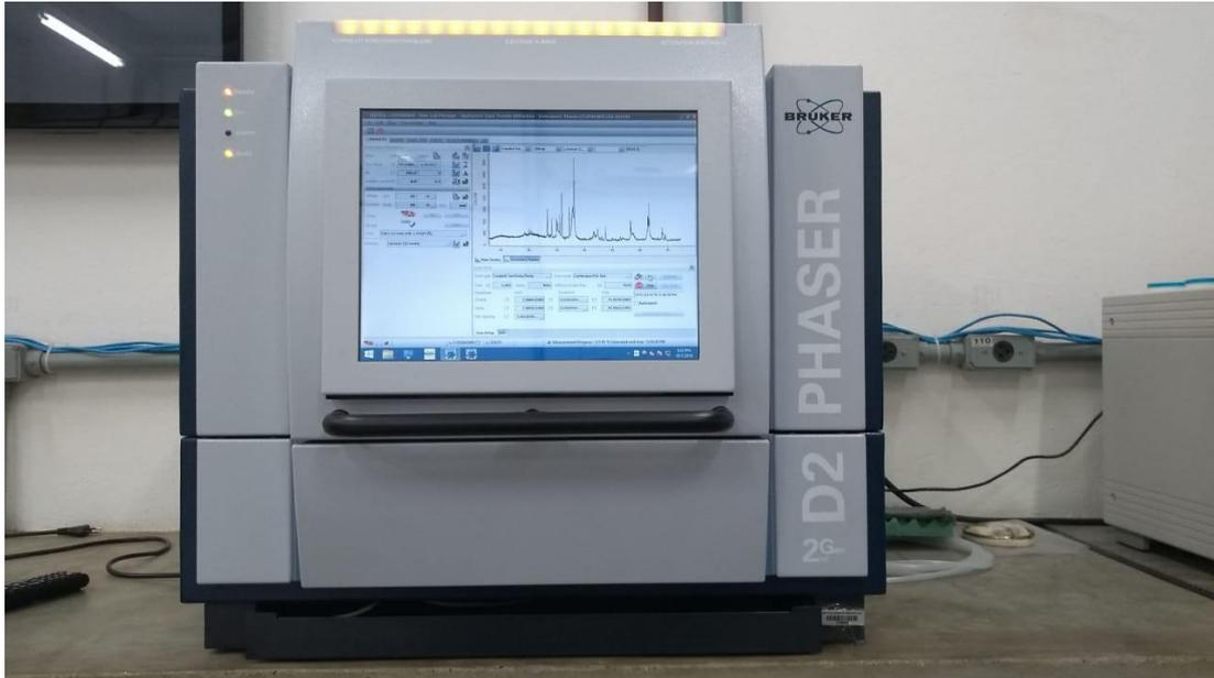
Figura 4.13 – DRX D2 Phaser, instalado no Nanolab (UFOP)
