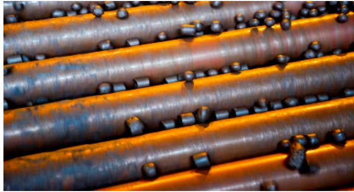
Figure 3.28. Cylindrical-shaped green pellets, evidencing their plastic deformation between rolls.
