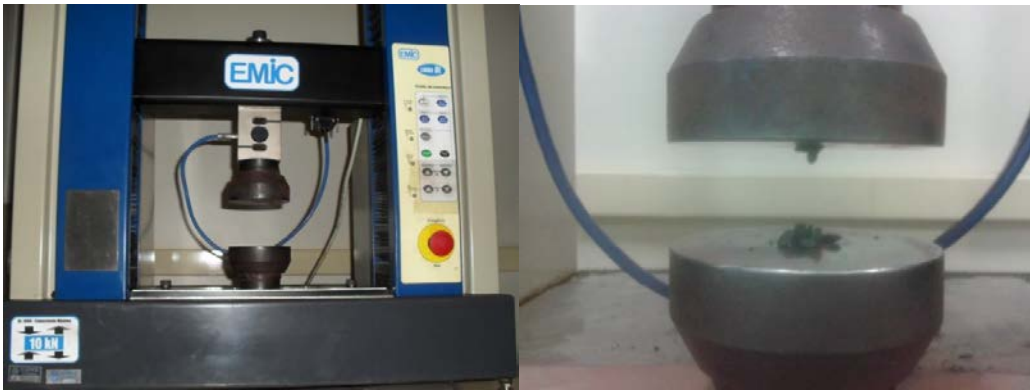
Figure 4.5. Compression test on EMIC 10 kN press.
