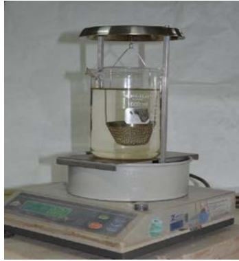
Figure 4.2. Hydrostatic density test setup.
