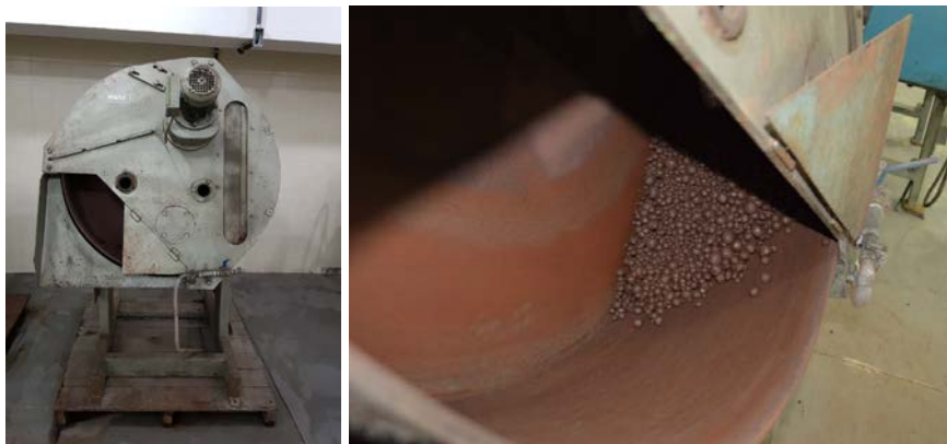
Figure 4.1. Eirich mixer used in green pellets preparation (left), and detail of green pellets produced (right).
