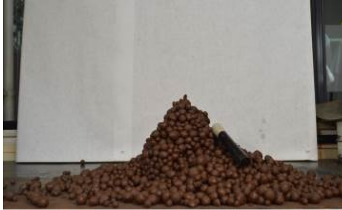
Figure 5.4. Repose angle test: final pile disposal profile.
