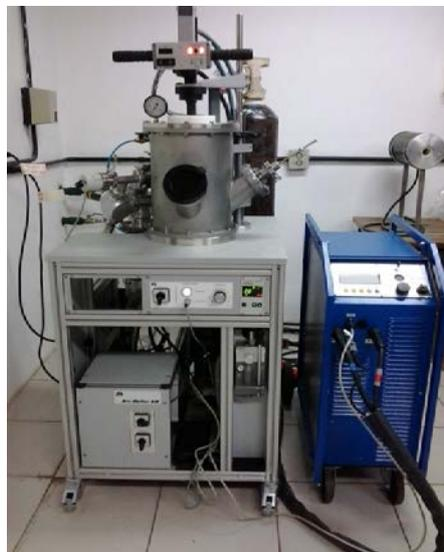
Figura 30 – Forno a arco Bühler AM-VARIO 400 [4].
