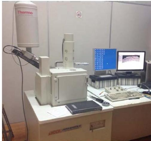
Figura 34 – MEV JEOL JSM 6460 (COPPE/UFRJ) [78].
