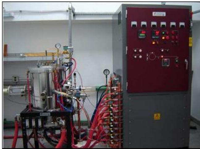
Figura 7 - Forno Series 45 Top Loaded Vacuum Furnaces (Centorr Vacuum Industries).
