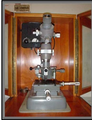
Figura 16: Microdurometro Ernest Leitz Wetzlar – Germany.
