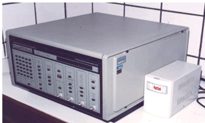
Figura III.1 – Potenciostato/Galvanostato modelo 273A da EG & G Instruments – Princeton Applied Research. [7]
