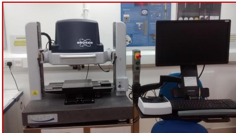
**Figura 33: Sistema de interferometria NPFLEX 3D**
