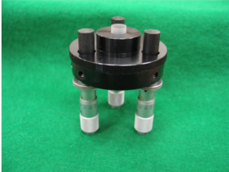
**Figura 3.10 – Tripod Polisher TM, modelo 590 da South Bay Technology Inc.**
